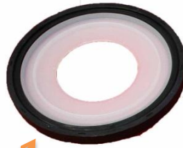
1 Seal with Shipping Protector Caution; Seal is reverse lip technology, blocking crankcase breathers during blowby measurement may cause oil leakage.
